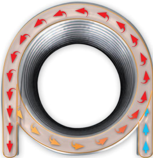
Ferrolì' research and engineering developed a heat exchanger which is simple and robust in its structure, using front-rank materials.
